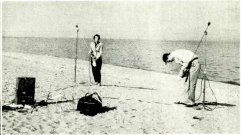
Left: James Bornemann adjusts one of the Telefunken mikes. Right: Handkerchiefs were tied over the microphones to cut down wind noise. The Telefunken's were spaced about 18 feet apart, parallel with the ocean, and back about 50 feet from the water.
