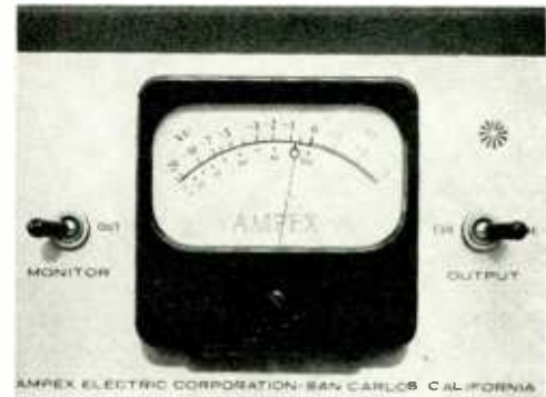
Above: When adjusting an alignment tape in a machine, care should be taken to reach the point of maximum output for the reproduce head, since a lesser peak will occur on each side of the maximum output position.
